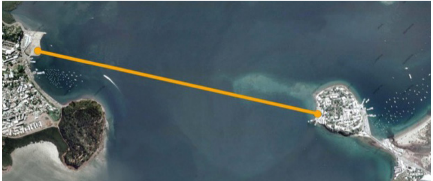
The project is a 2.5 Km pipe of fresh water in coral seafloor (© Google Maps)
